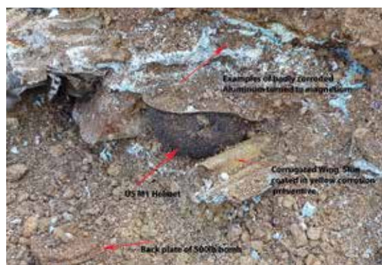
(Fig. 10.3) — Corrosion effects on iron artifacts versus aluminum (Photo P. Murphy © WWIIBRPG).
