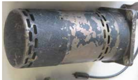
(Fig. 6.3) — Amplidyne 28/60vlt motor at the General Patton Memorial Museum (Photo P. Murphy © WWIIBRPg).
