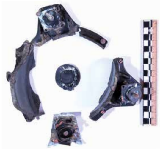
(Fig. 15.1) ____ Flux Gate Gyro transmitter- Bendix Corp located in the left wing.
