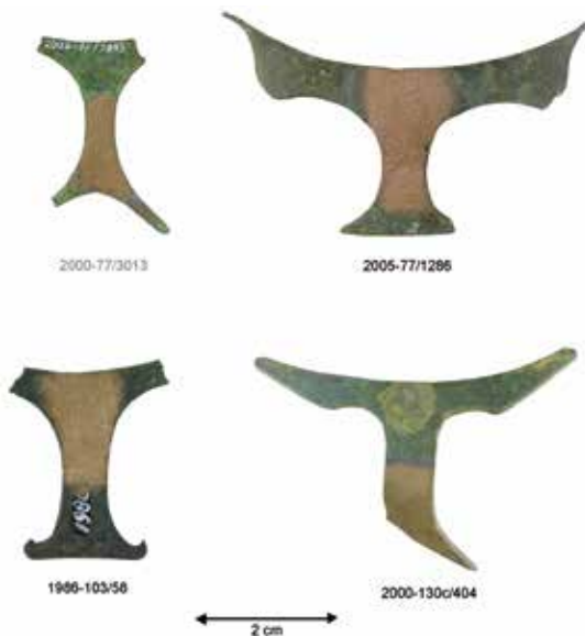
(Fig. 6) — Thumb plates found on the Titelberg showing the corundum blasted spots used for performing the XRF analysis.
