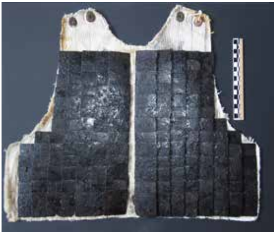
(Fig. 17.1) ____ State-of-the-art designed upper Flak vest, containing magnesium-iron plates and first- generation Nylon Kevlar type material, before and after restoration (P. Murphy © WWIIBRPG).
