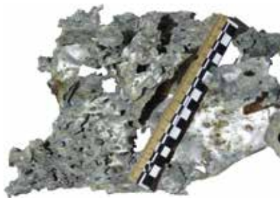
(Fig. 13.2) — Frontal flak damage to an engine cover (P. Murphy © WWIIBRP6).
