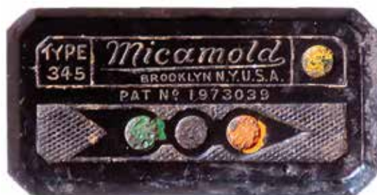
(Fig. 15.4) ____ Color-coded capacitors in radios and electrical systems (P. Murphy © WWIIBRPG).
