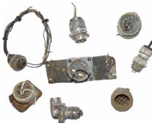
(Fig. 15.3) ____ Amphenol-Cannon plugs, still used unchanged today (P. Murphy © WWIIBRPG).
