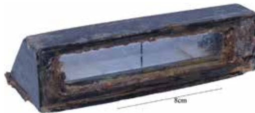
(Fig. 14.5) — The Sherman tank periscope head, M3 or M4, 2021-034/294, USBC-007 (P. Murphy © WWIIBRPG).
